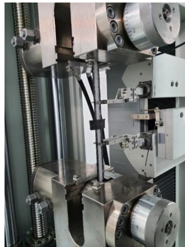
Figure 3.9. The view of the tensile test of the geogrid
