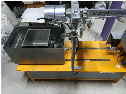
(a) Outer chamber in specimen preparation station
