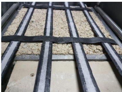
(g) Geogrid placement on the shear surface
