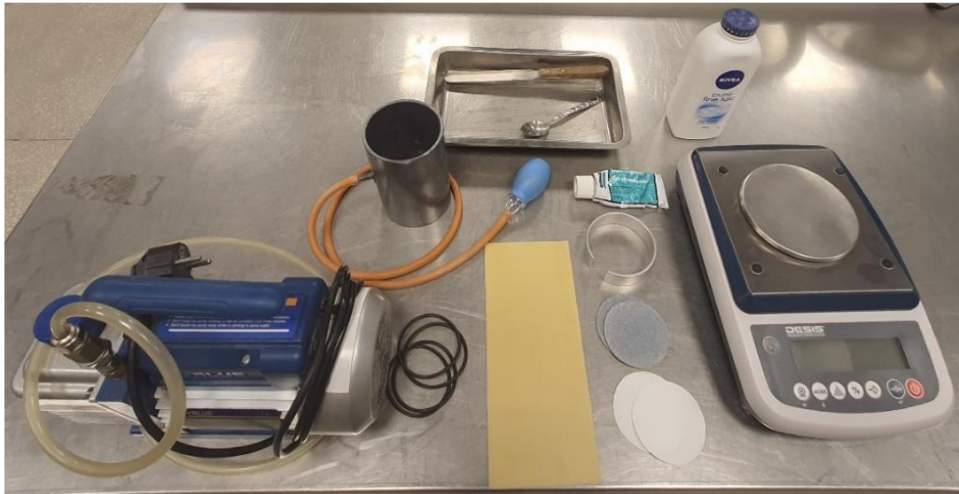
Figure 3.14. Apparatus for flexible wall hydraulic conductivity testing of CFM
