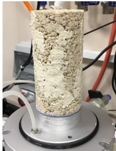
Figure 3.19. Coating of the large gaps with a thin layer of moistened kaolin clay
