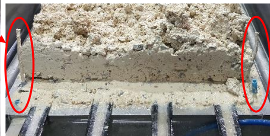
(d) Position of the perforated pipes at the corners of the upper box at the end of the shear test
