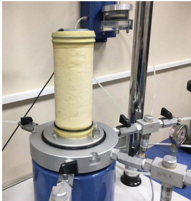
Figure 3.20. Sealing the specimen between the top and bottom plates with O-rings
