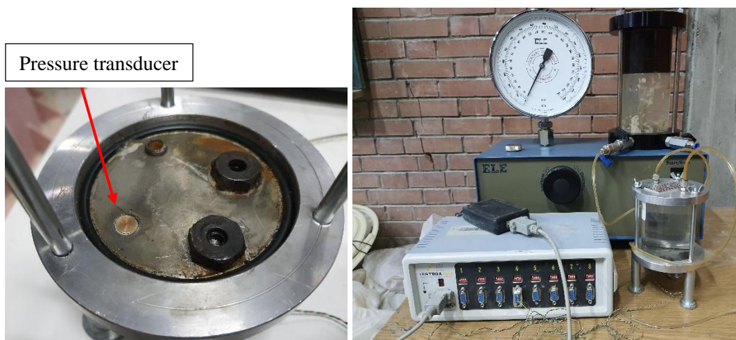
Figure 3.45. Calibration of the pressure transducer
