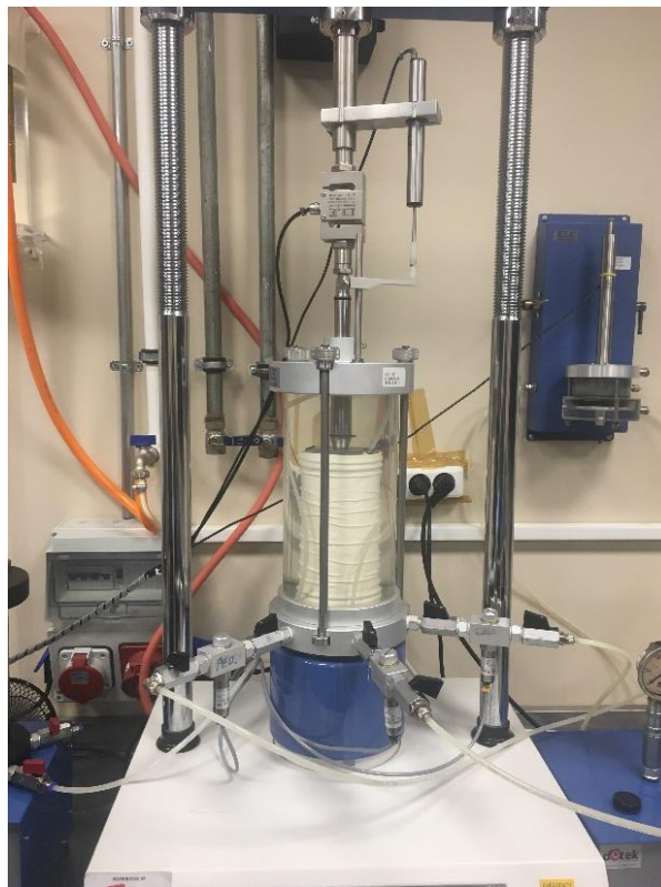
Figure 3.24. Loading frame and the cell for triaxial compression tests
