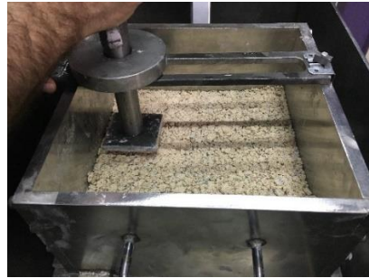
(b) CFM compaction in layers
