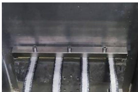
(e) Geogrid fixing to the clamping mechanism
