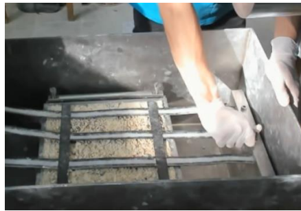
(f) Fixing the geogrid
