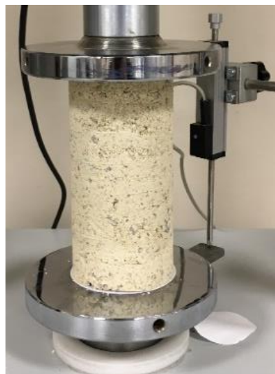
Figure 3.22. Placement of the specimen to the unconfined compressive strength equipment
