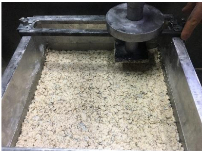
(e) CFM compaction in the lower box
