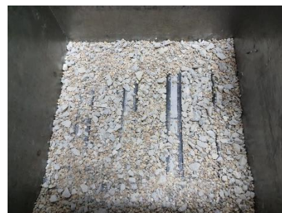
(f) Specimen placement in the upper box
