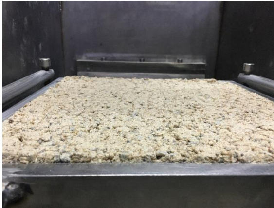
Figure 3.35. Soil surface protruding from the lower box level on which the geogrid will be placed
