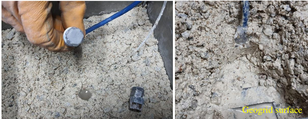
Figure 3.46. (a) Placement, and (b) vertical position of the pressure transducer within the compacted specimen
