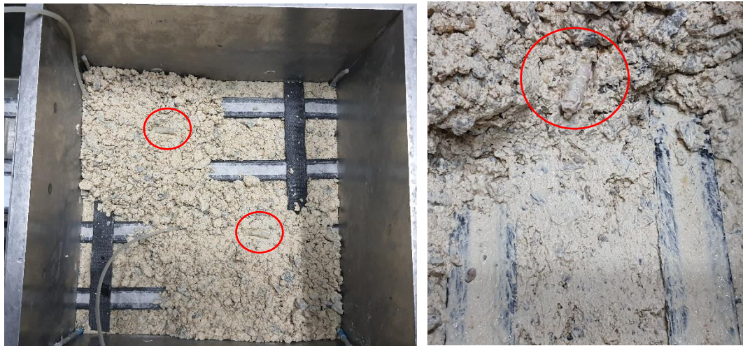
(a) Horizontal positions of piezometer pipes (b) Vertical position of piezometer pipes
